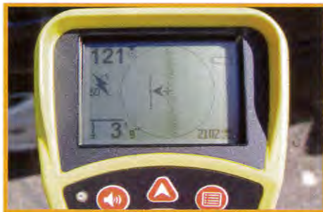
Distorted signal, caused by the large metal car parked over the conductor's path.
